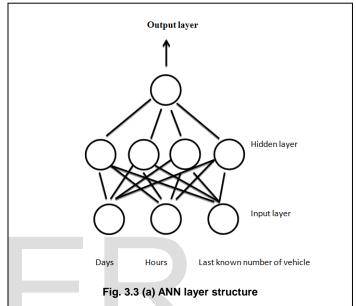
to predict data set with the three layers of the model. But the ANN algorithm has also trained with python on the collected data to give illustration graphically for traffic flow prediction with a time interval of one hour. In this way, a user may check traffic flow prediction by using the system.
