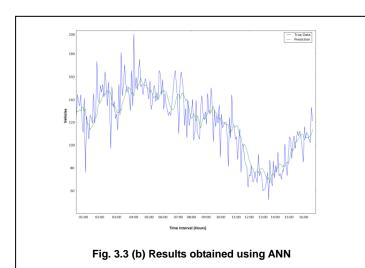
using the ANN model having two lines blue lines shows the true data, which means original data collected from PEMS. And green lines show the predicted data that we have after applying the ANN algorithm on the existing data.
